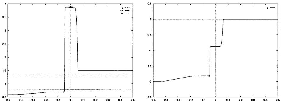
FIG. 6. Propagating phase boundary. (a) Volume component; (b) velocity component.
