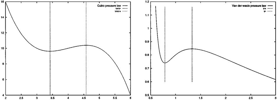
FIG. 1. (a) Cubic pressure law; (b) van der Waals pressure law.
