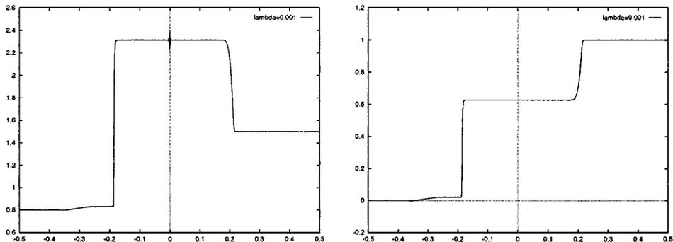
FIG. 11. Nonclassical shock wave (Van der Waals). (a) Volume; (b) speed.
